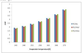
Fig: 2. Variation of COP with evaporators'
