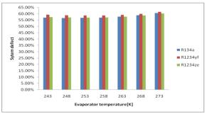
Fig: 4. Variation of system defect with evaporator temperatures
