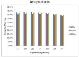
Fig: 3. Variation of exergetic efficiency with evaporators' temperatures
